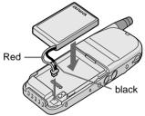
Orient the connector as shown.
